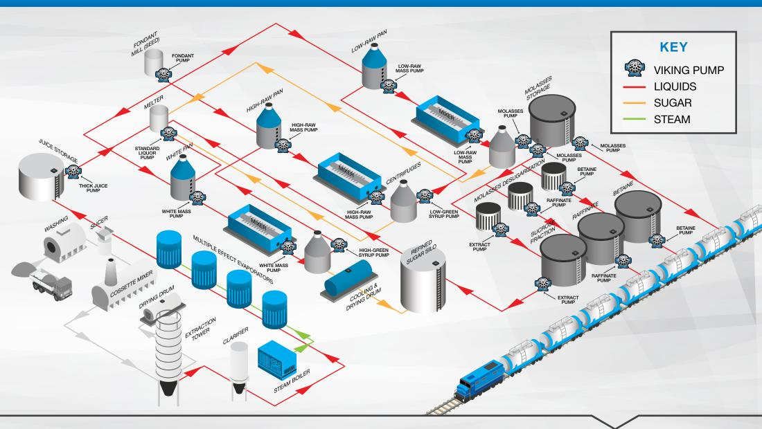
In beet plants, Viking pumps are typically found downstream of the evaporators – on thick juice, standard liquor, white pan massecuite, high-green syrup, high-raw massecuite, low-green syrup, low-raw massecuite, molasses, sucrose extract, betaine and raffinate, as well as metering fondant and processing liquid sugars and inverts. They are used in 24/7 process applications as well as loadout applications to packaging, trucks and railcars.
