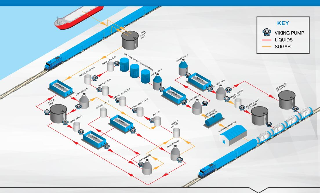
Viking pumps are found throughout the process of refining raw sugar into finished sugar and liquid products. Applications include affination syrup, magma, fine liquor, massecuite, refiners' molasses, liquid sugar and invert.
