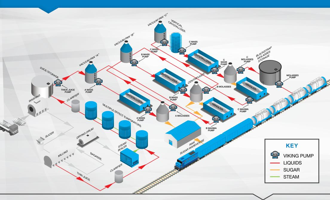
In cane mills, Viking pumps are typically found downstream of the evaporators – on thick juice, "A, B & C" massecuite, "A, B & C" molasses, magma, and on imported cane juice molasses.
